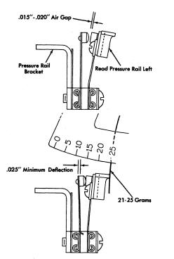
Figure 128. Contact Adjustment
