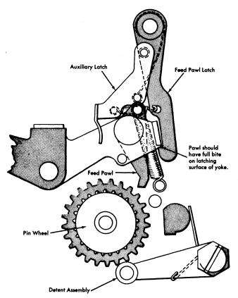
Figure 122. Feed Pawl Latch Bit
