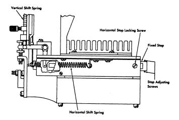
Figure 84. Print Interposer Assembly
