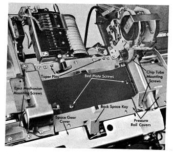
Figure 45. Punch Bed (Front View)
