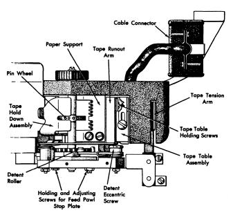
Figure 120. Tape Registration Adjustment
