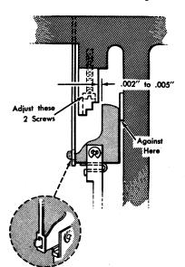
Figure 55. Pin Latch Stop
