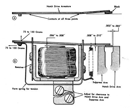
Figure 59. Notch Drive Magnet
