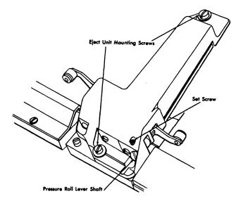
Figure 29. Master Station Registration Adjustment
