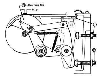
Figure 67. Stacker Adjustment
