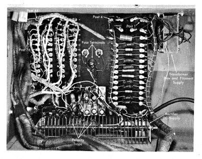
Figure 1. 24-Base Power Supply (Old Style)
