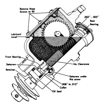
Figure 11. Reduction Drive Adjustment
