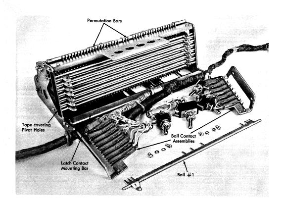
Figure 92. Keyboard Permutation Unit
