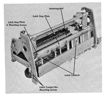
Figure 93. Keyboard Permutation Unit
