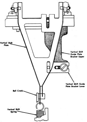
Figure 82. Code Plate Adjustment
