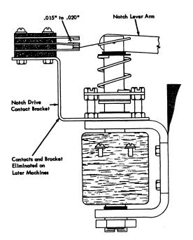
Figure 62. Solenoid Drive Unit
