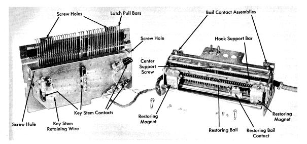
Figure 95. Keyboard Permutation Units
