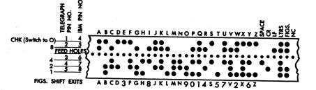
Figure 105. Telegraph Printer Code
