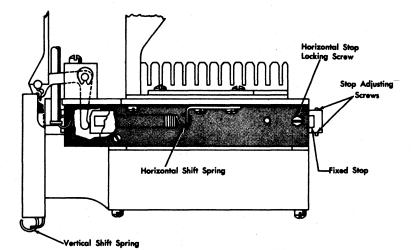
Figure 81. Print Interposer Assembly
